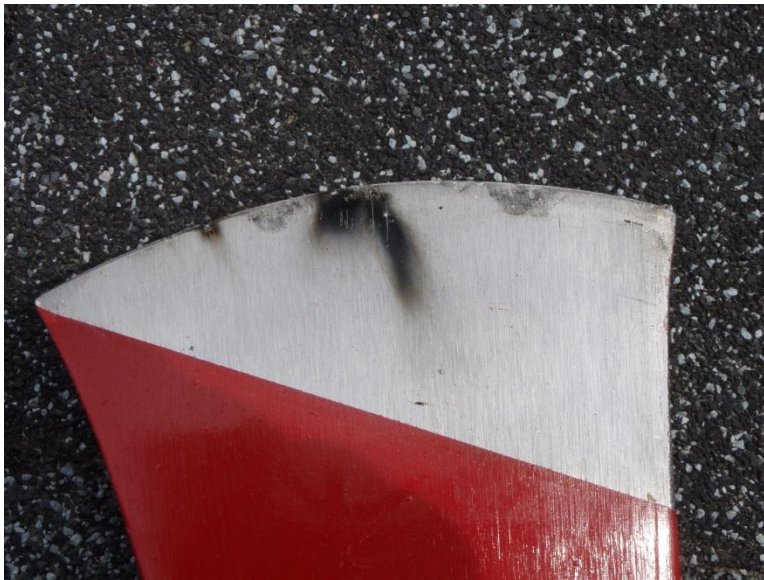
Figure 52 Carbon deposit from arcing on axe blade after severing conductor
