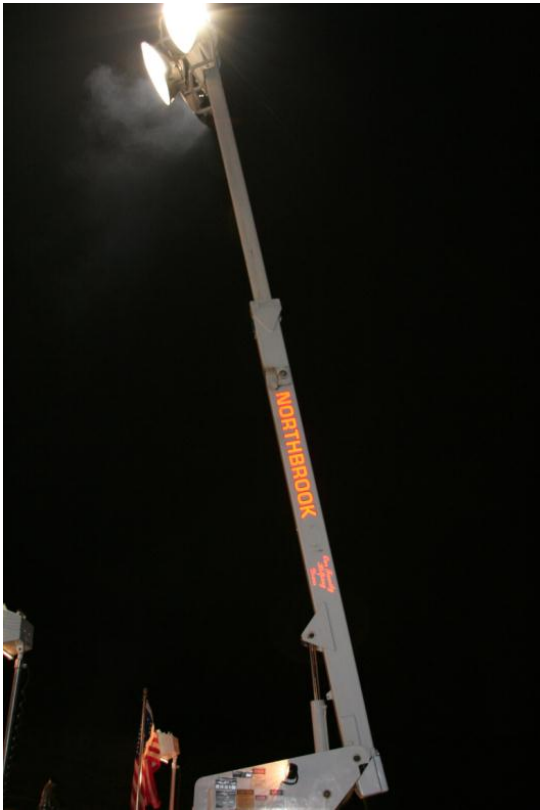
Figure 71 Light Truck No. 2 boom lights
