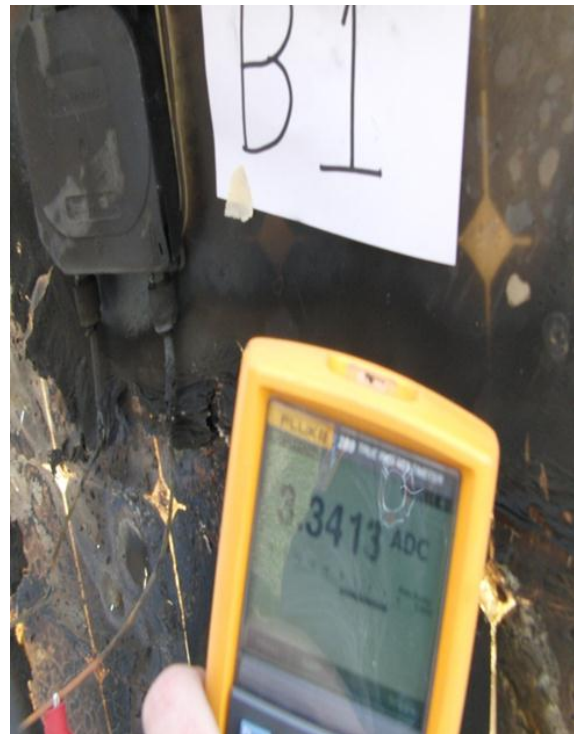
Figure 116 Module B1 – damaged but still producing over 3 amperes
