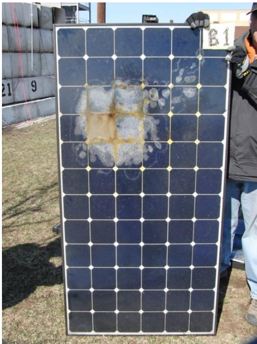
Figure 116 Module B1 – damaged but still producing over 3 amperes
