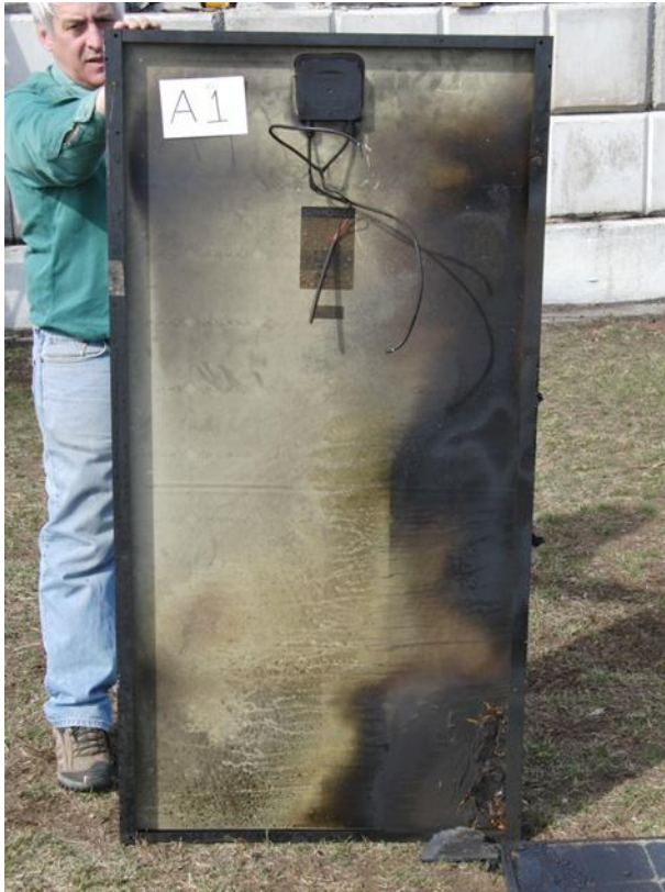
Figure 115 Module A1 – damaged but functional and producing full voltage
