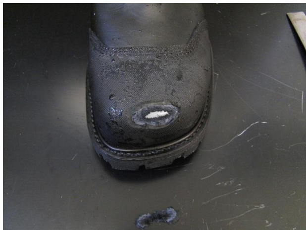
Figure 37 Boot #3 with material removed
