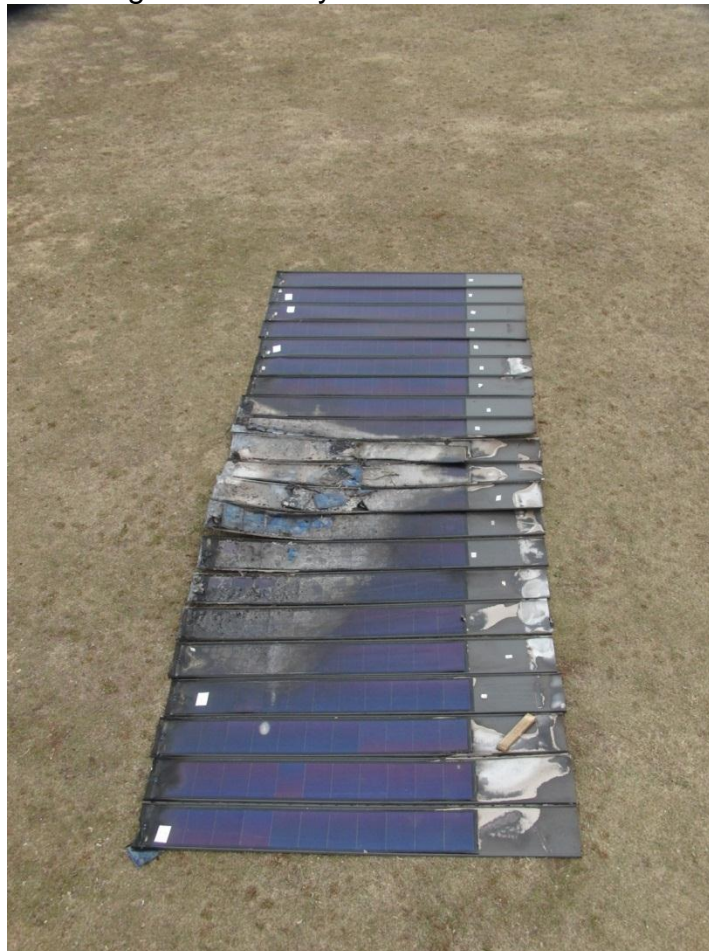
Figure 141 Array reconstructed on ground, post-fire
