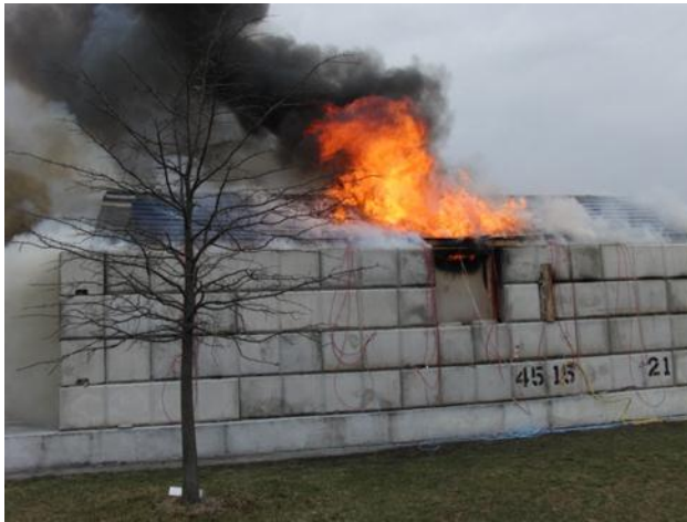
Figure 146 Solar shingles on fire
