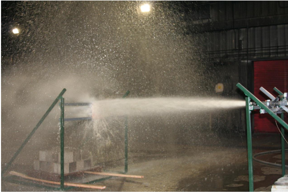
Figure 8 Water stream aimed at energized target plate
