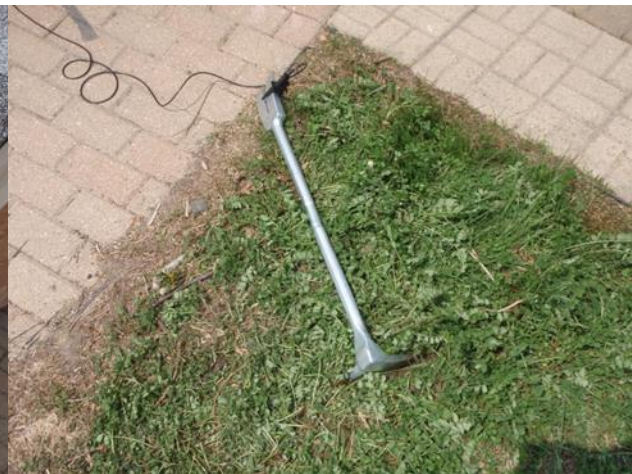
Figure 66 Halligan tool imbedded in ground
