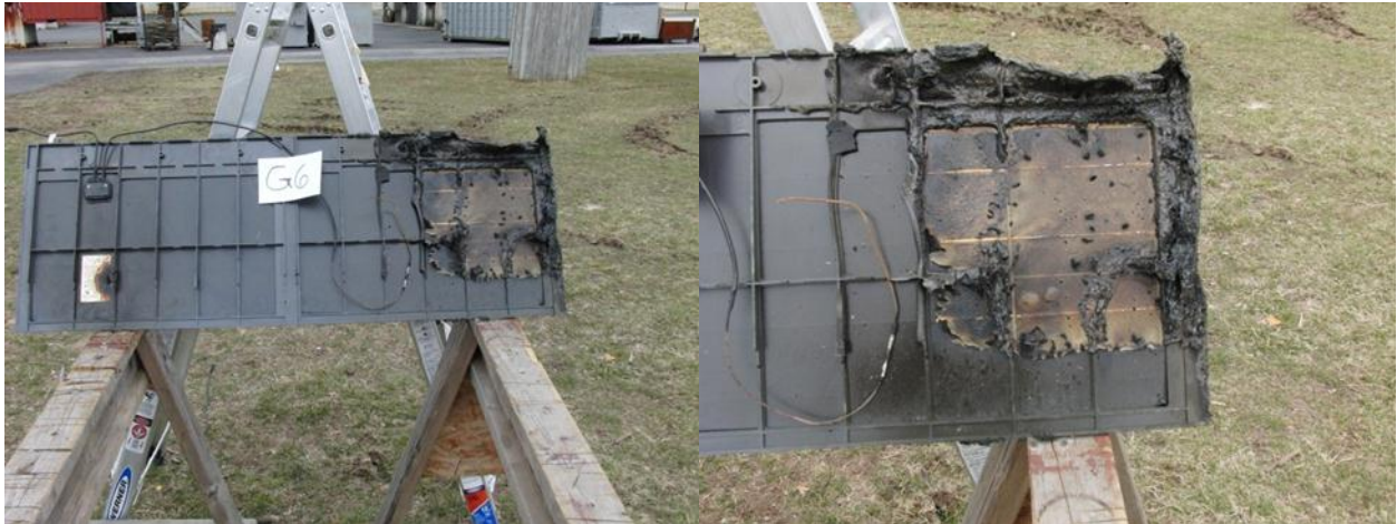
Figure 160 Damaged shingle G8, exposed conductors and bus - fully functional
