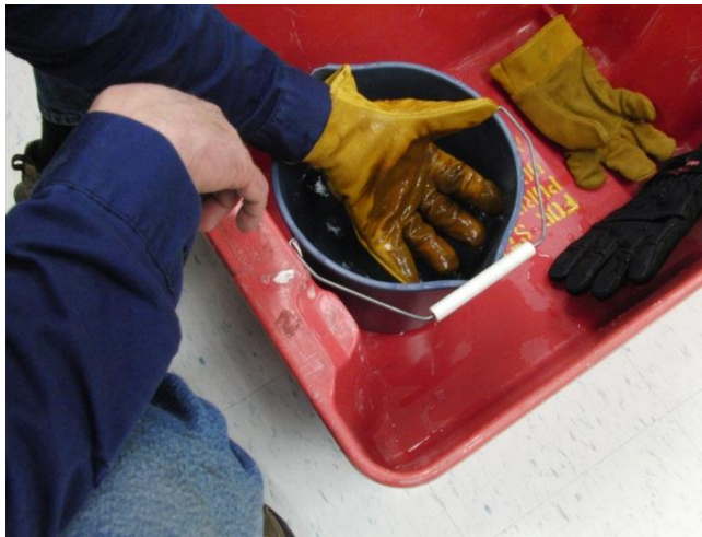
Figure 30 Wetting a glove before test
