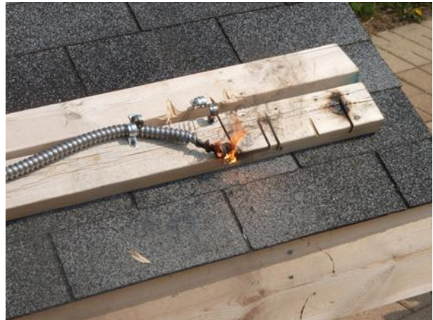
Figure 59 Open flame from arcing
