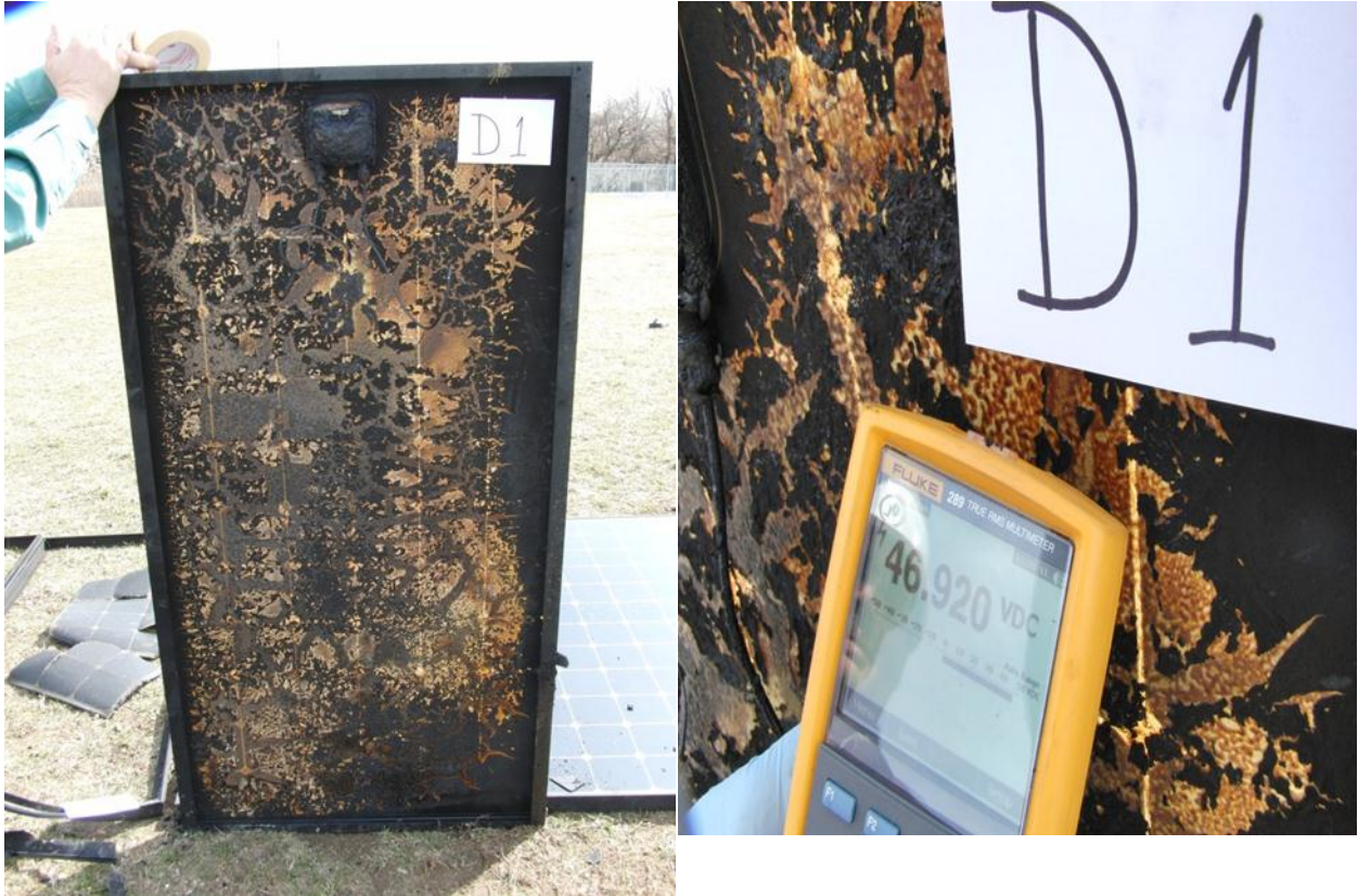
Figure 117 - Module D1 – badly burnt on backside, but functional and producing full voltage
