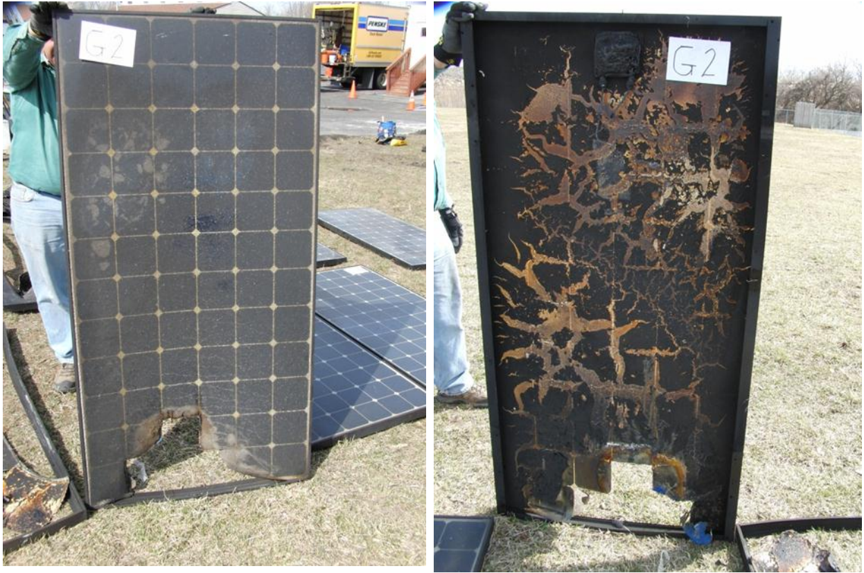
Figure 118 Module G2 – bottom portion of module glass and cells destroyed
