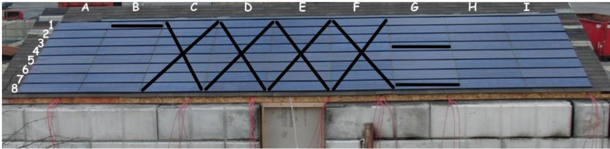
Figure 155 Roof diagram after fire test: “X” or “-” represents no power
